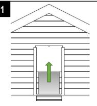
Raise the sliding door to its fully open position.
