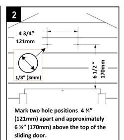
Make sure they are level and evenly spaced above the centre of the door. Make the holes with a 1/8" (3.0mm) drill bit or bradawl.
