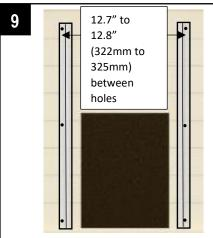
Once the channels are vertical and the holes 12.7" – 12.8" (322mm – (325mm) apart, mark the locations for the six fixings. Drill 1/16" (1.5mm) diameter holes.
