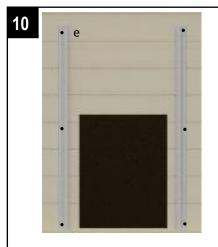
Fit the channels with the six black wood screws (e).
