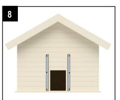
Position the channels on each side of the door hole on the hen house with the hole central between the channels. They must be perfectly vertical, flat and level. The fixing holes must be 12.7" – 12.8" (322mm – 325mm) apart.
