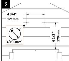
Mark two hole positions 4 ¾" (121mm) apart and approximately 6 ½" (170mm) above the top of the sliding door.
