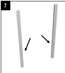
The channels are fitted to the hen house with the rivets at the bottom of each channel, not nearer to the top.
