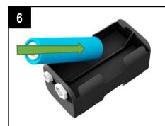
Fit the batteries into the holder.
