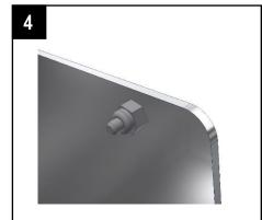
Tighten each nut by turning the screw with a screwdriver whilst holding the nut with pliers or a wrench.
