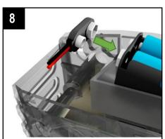
Fit the connector to the battery holder.
