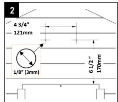
Mark two hole positions 4 %" (121mm) apart and approximately 6 %" (170mm) above the top of the sliding door.
