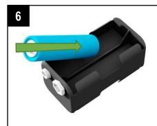
Fit the batteries into the holder.
