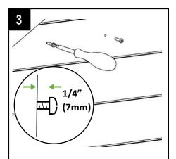
Start to fit the two screws supplied into the holes you have made.
