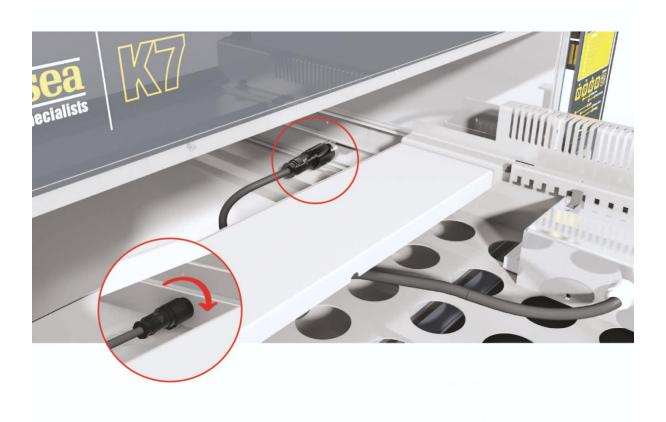
Gently lower the turn system floor onto the chassis. The toothed rack must fit over the side of the motor pinion, the floor will align itself once lowered into place.
