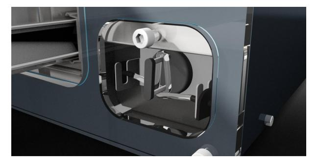
The tube that is held around the pump capstan is of precise length to ensure it is correctly "pinched" where it rolls on the capstan pins. It will wear out during extended use and should be replaced periodically with a new length of tube 110mm long. This length is shown below for reference:
