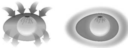
Comparison of heat flow in naturally and artificially incubated eggs
