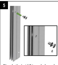
Fit a plastic rivet (d) to each channel in the hole shown.
