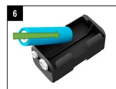
Fit the 4 batteries into the holder.
