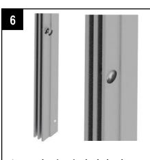
Locate the rivet in the hole, then push it in to secure it.
