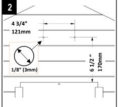
Mark two hole positions 4 %" (121mm) apart and approximately 6 %" (170mm) above the top of the sliding door.
