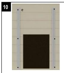
Fit the channels with the six black wood screws (e).
