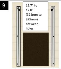
Once the channels are vertical and the holes are 12.7" – 12.8" (322mm – 325mm) apart, mark the locations for the six fixings. Drill 1/16" (1.5mm) diameter holes.
