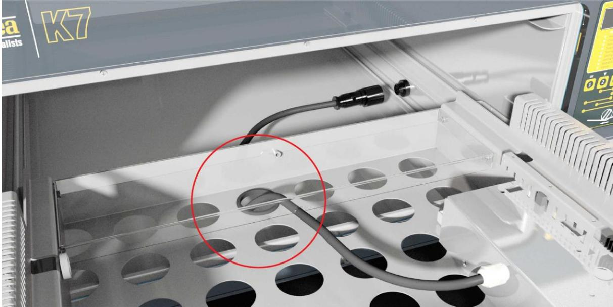
Lower the turn system chassis down into the drawer so that it locates centrally over the centre guide pegs. Correct location is important, the assembly will rock from side to side to show if it has not been fitted correctly and needs to be repositioned.
