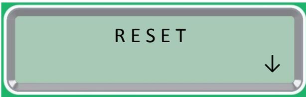
This screen shows during setup if the system detects an error after the batteries are connected for the first time.
